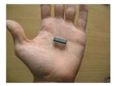
MAX232 is an incorporated circuit that changes over signs from a RS-232 serial port to flags suitable for use in TTL perfect advanced rationale circuits.
