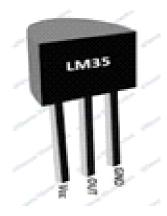
The LM35 is a coordinated circuit sensor that can be utilized to gauge temperature with an electrical yield corresponding to the temperature (in oC).
